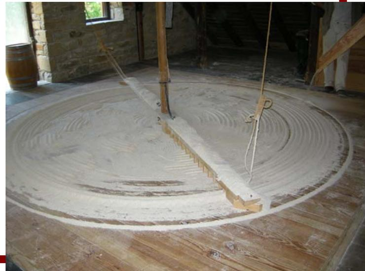
Sifting occurred on the second floor and the hopper boy was located on the top level of the three and a half storied stone structure. This is a fully operational Oliver Evans mill that operates today using reproductions of the original machinery. Paid personnel are used to operate the mill.
